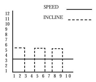
The **Fat Burn Program** is designed to vary the treadmill elevation, while maintaining a constant walking belt speed.
